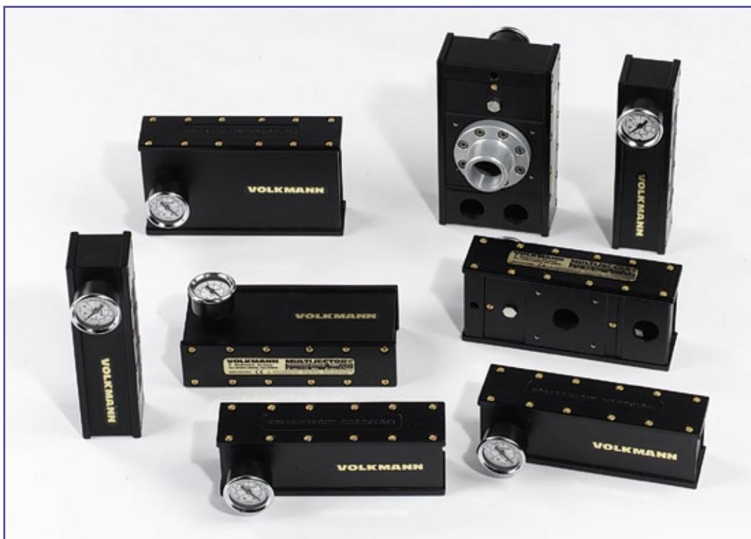
Multipoint pumps of the M- and ML-series work with **three ejector stages** which are connected in a row. Their robust and compact aluminium casing makes the pump resistant even to strong mechanical or thermal loads. Nevertheless they are very light and offer considerable amounts of suction air at a small size. The compact form allows them to be mounted directly at the location where vacuum is needed.
