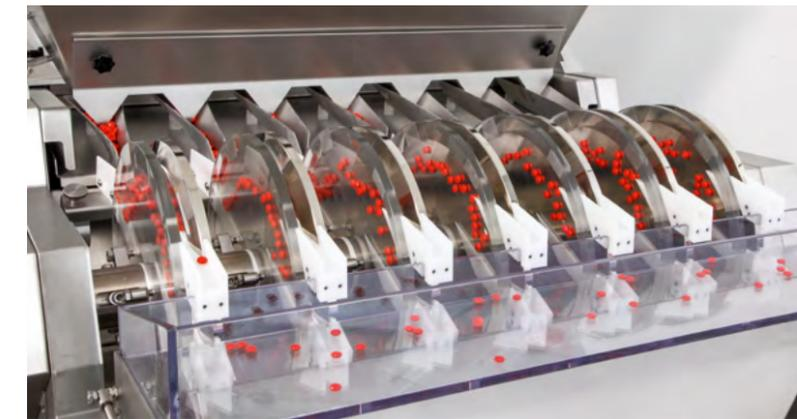
The Bohle Tablet Checker is used for a mechanical check of the thickness of sugar-coated or film-coated pills, capsules and tablets.
