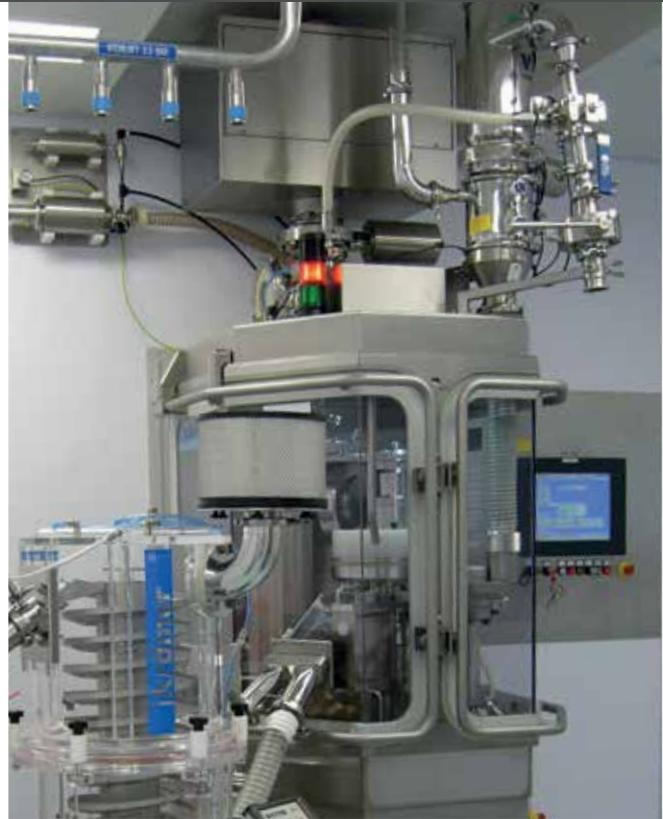
PPC (WIP) for charging a tablet press.
