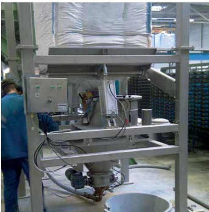
The big bag emptying station in the construction industry with massagers and lump breaker for products which do not flow easily.
