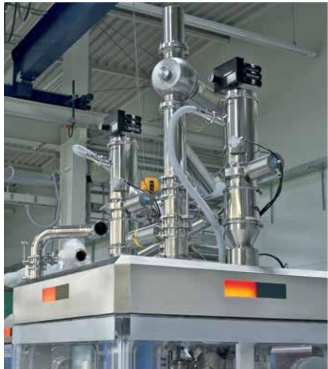
PPC with a WIP function on a table press.
