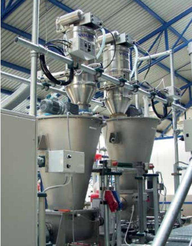
Two vacuum conveyors for loading loss-in-weight feeders.
