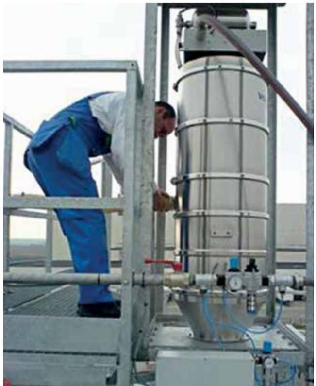
Vacuum conveyors in an outdoor installation, for charging silos.
