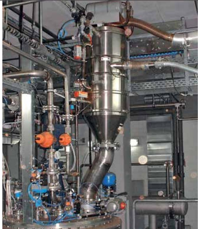
Vacuum conveyor with a powder lock for conveying pigments in a solvent atmosphere.
