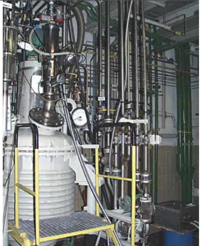
With VOLKMANN INEX vacuum conveyors, material can be simply and safely transported in hazardous processing systems such as stirred tanks and reactors. This enables powder to be transferred in all dust and gas explosion zones.
