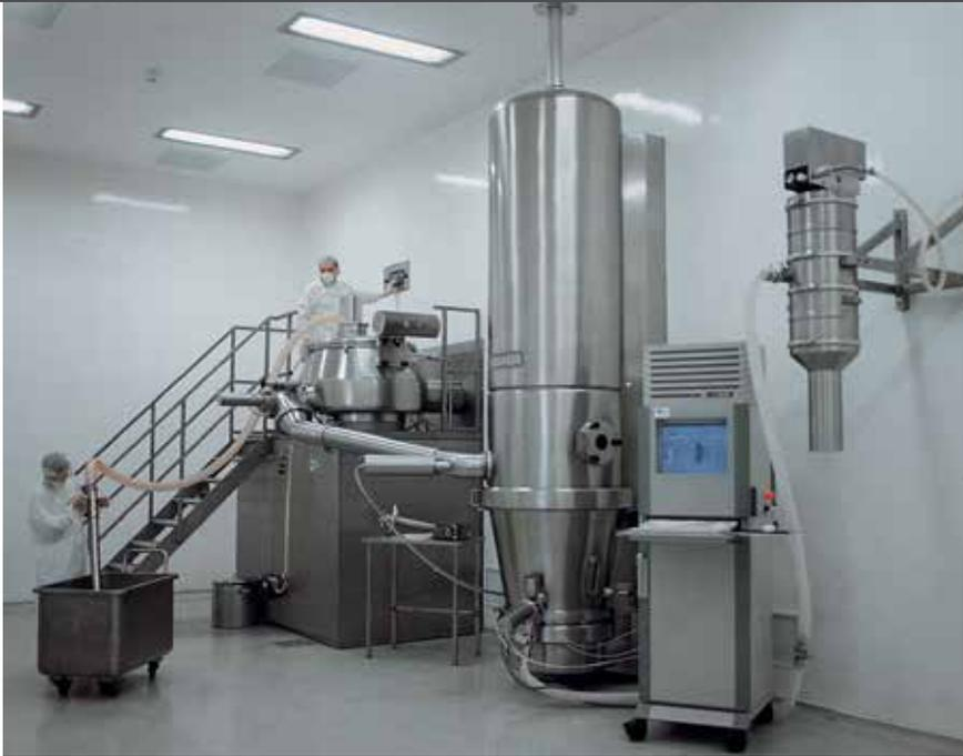
Vacuum conveyor for automatically emptying a fluidized bed dryer.
